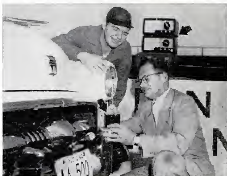
Mounted on bumper is the test transmitter of timer unit (arrow). Top arrow points to receiver unit. New design is much smaller
